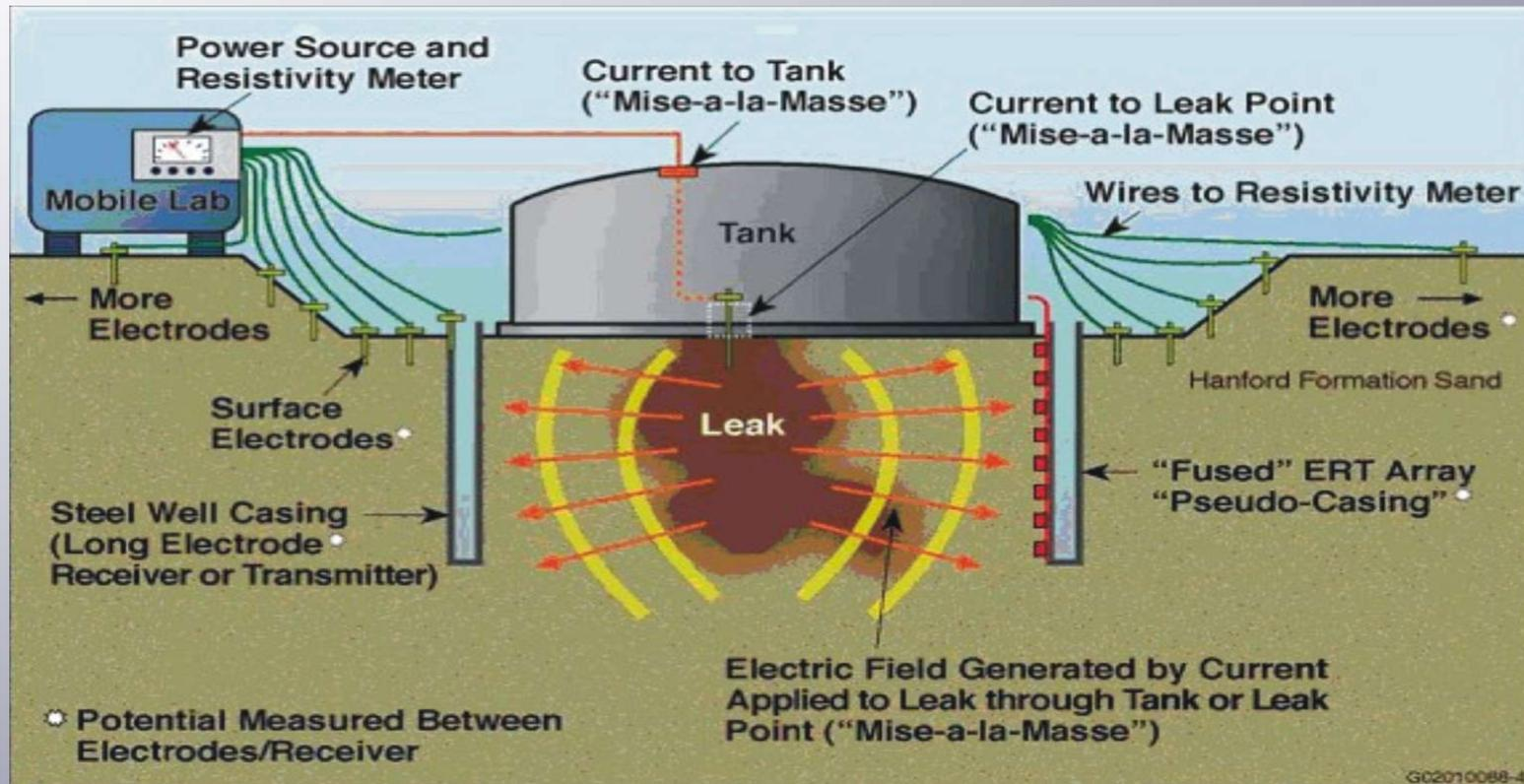
*The Monitoring Program Takes Advantage Of Changes In Contact Resistance That Will Occur If Conductive Tank Liquid Leaks Into The Soil.*
