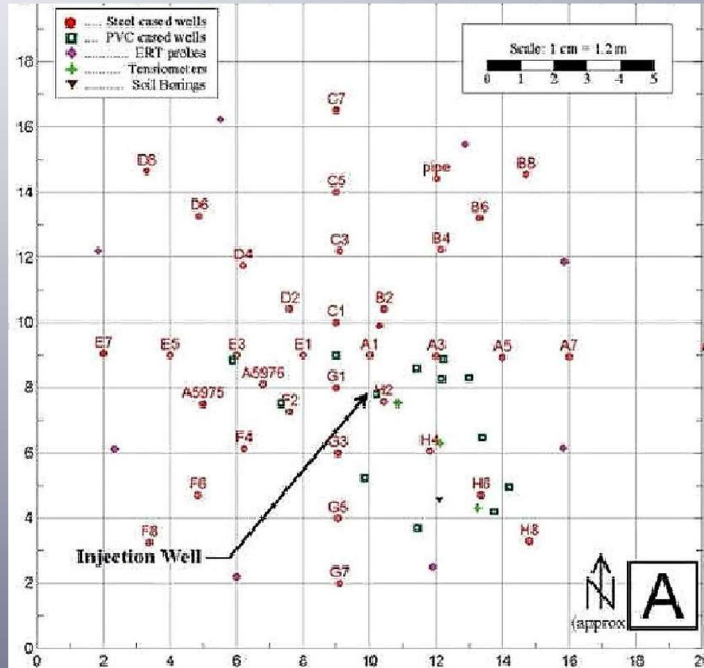
layout of steel-cased monitoring wells and injection well
