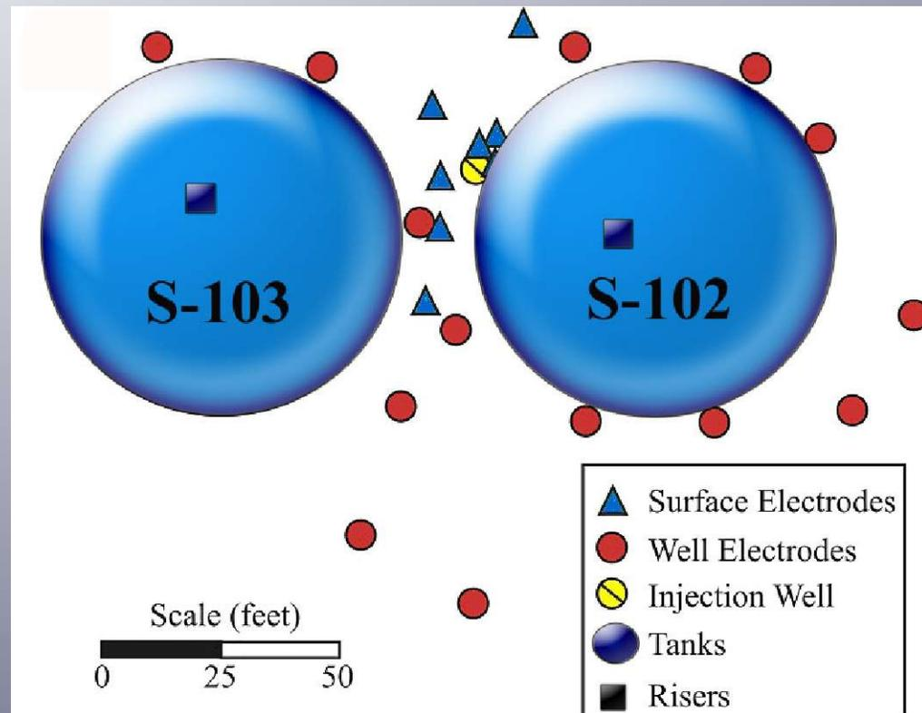
Layout of LDM electrodes & injection well for
